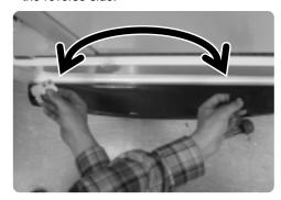
After removing the left and right side screws, disassemble the Grommet, Stopper Door and Stopper-Mid of the right bottom of freezer-door.
